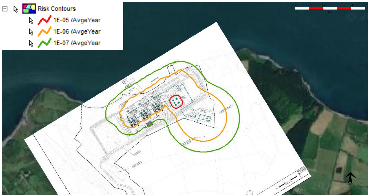
Figure 12 Outdoors Individual Risk Contours with plot plant
