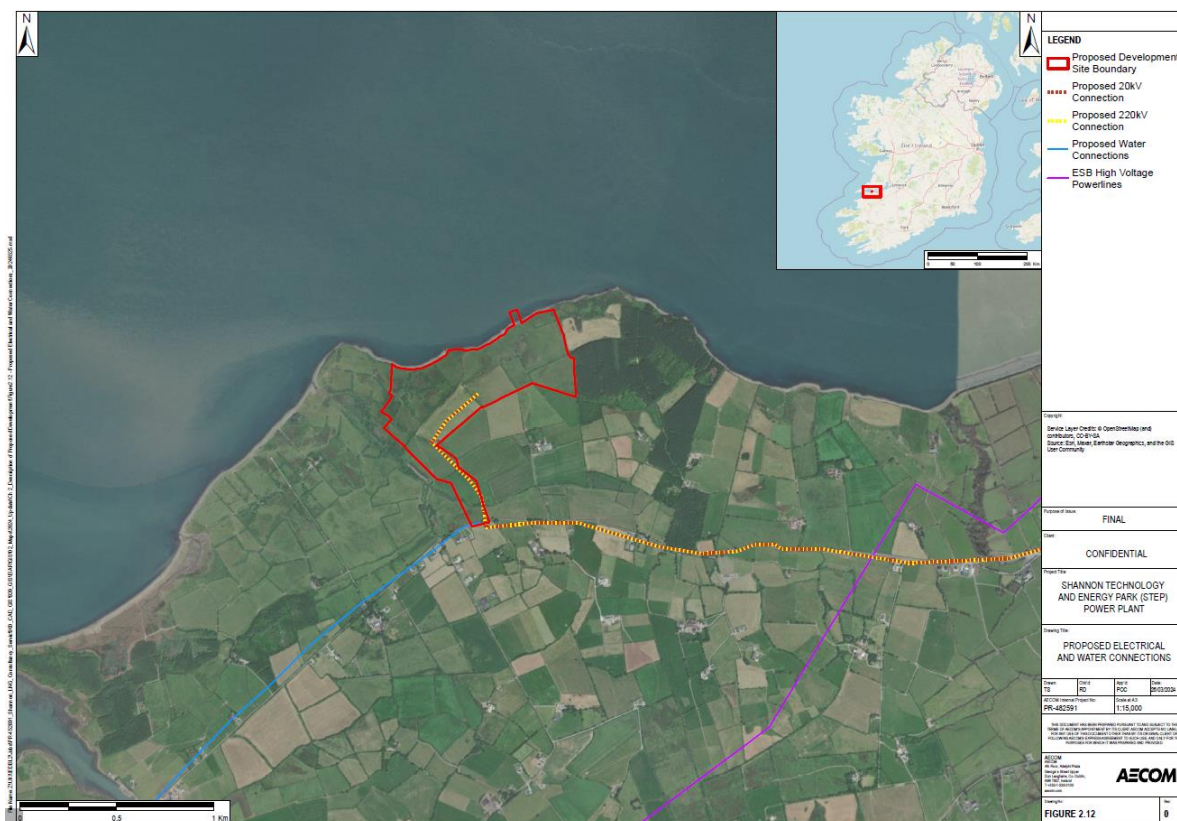
Figure 2.12 Proposed Electrical and Water Connections
